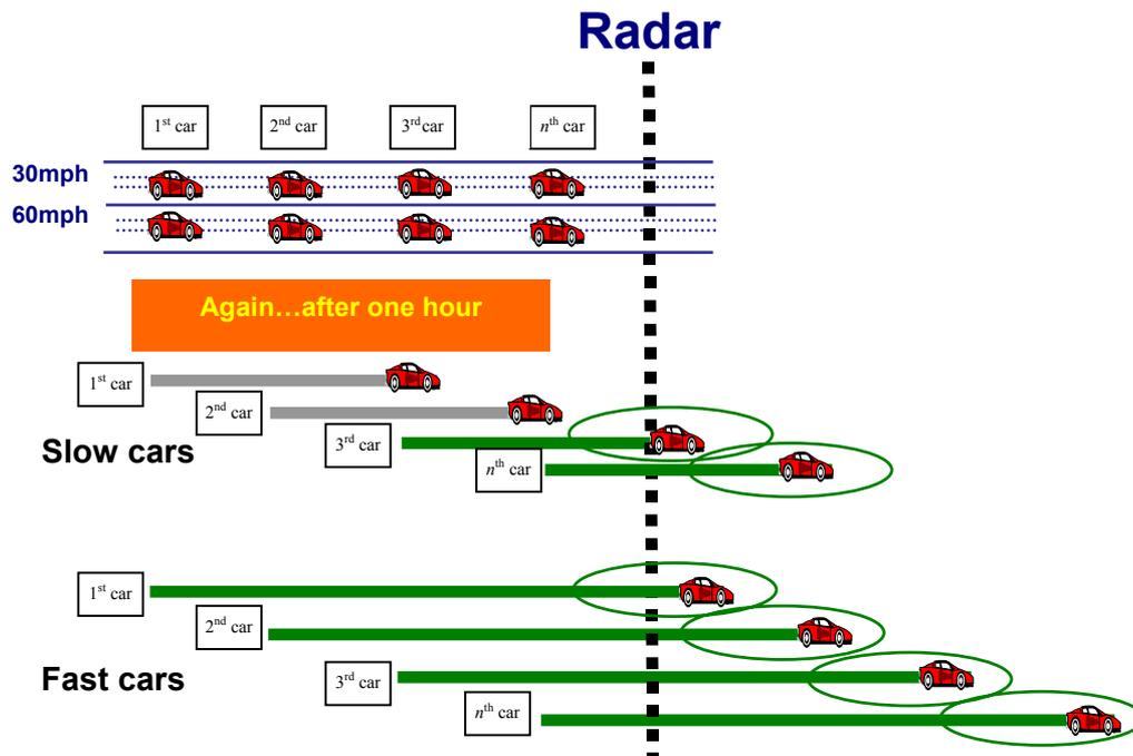
**Figure 3** A radar gun measures the speeds of fast and slow cars that pass its location during an hour. The number of recorded (circled) cars is proportional to their speed.
