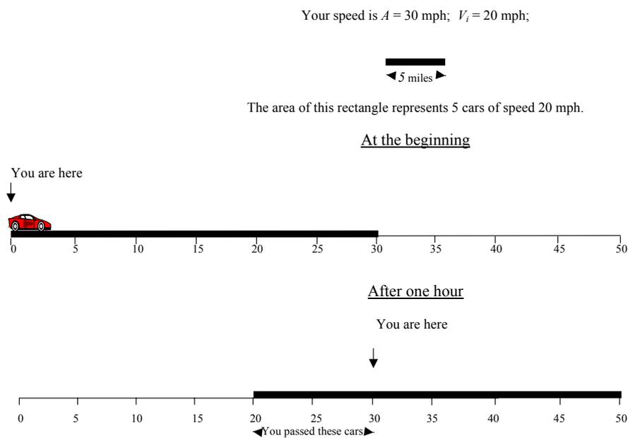
**Figure 2 The positions of your car, and of all the cars that drive 20mph within a range of 30 miles, at two points of time, one hour apart.**
